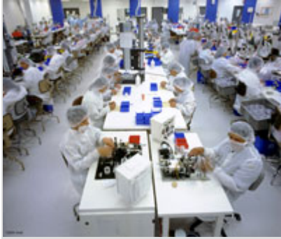
Single-use device assembly in one of Avail's state-of-the-art Mexico clean room facilities. Photo courtesy of Avail.
