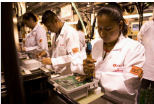
Workers assemble printed circuit boards for medical device and other OEMs in Guadalajara, Mexico. Photo courtesy of Solectron Corp.
